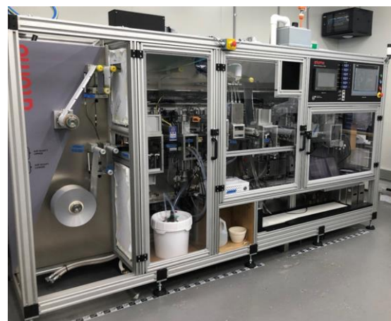
Atomo's Next Gen High volume blister manufacturing machine
